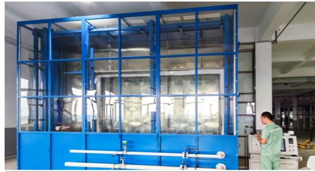
门窗气密、水密、抗风压性能 实验室检测室检测设备 Air tightness, water tightness and wind pressure resistance of doors and windows Testing Equipment for Laboratory Testing Room
