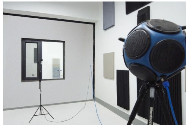
门窗空气隔声性能检测 Air sound insulation performance test of doors and windows
