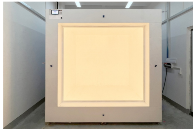
门窗采光性能检测设备 Detection equipment for lighting performance of doors and windows
