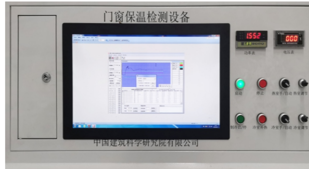
门窗保温性能检测设备中控台 Center console of door and window thermal insulation performance testing equipment
