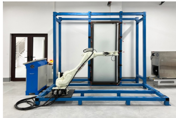
门窗耐久性能机械手检测设备 Mechanical arm detection equipment for durability of doors and windows
