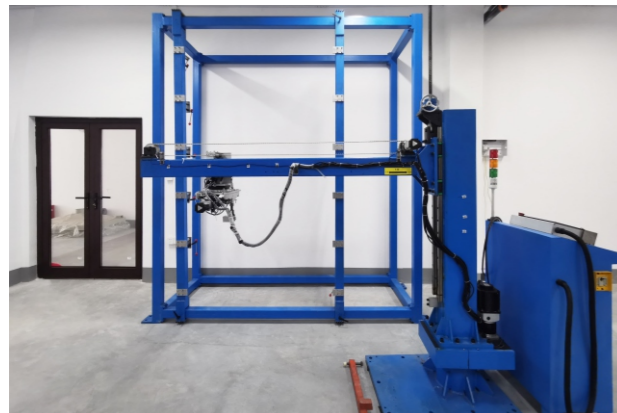
门窗耐久性能单臂式检测设备 Single arm type testing equipment for durability of doors and windows
